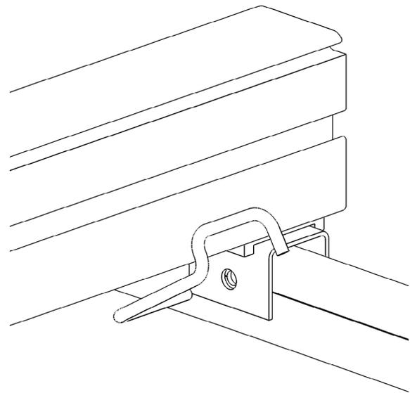
3. Rotate the G-Clip downward to lock into position
